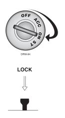
If power door locks have been connected to your system, the vehicle's door will lock three seconds after the ignition has been turned on and unlock when the ignition is turned off.
